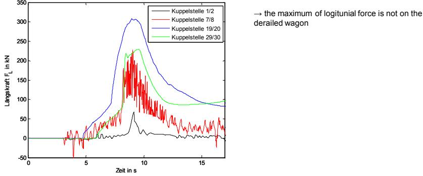
→ the maximum of longitudinal force is not on the derailed wagon
