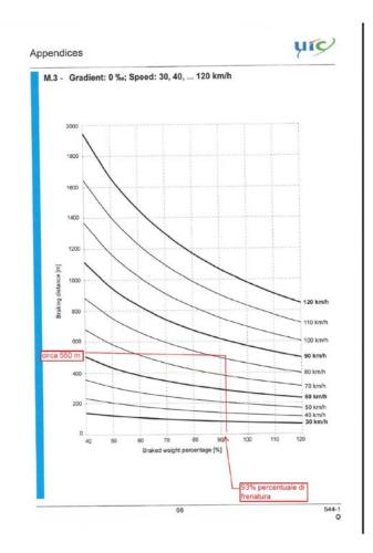
The calculation of the braking distance (550 m) was obtained by considering
