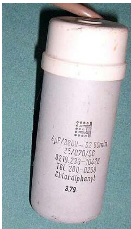
Capacitor containing PCBs
