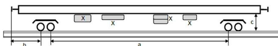
A: Defined distances and areas (the illustrated bogies with two axles are only an example; a bogie can consist of different numbers of axles)
