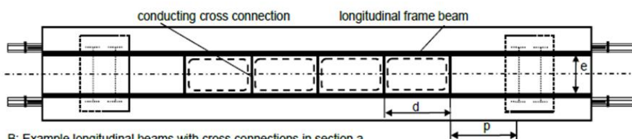
B: Example longitudinal beams with cross connections in section a
