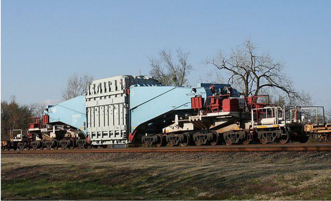
Figure 1: Example of a vehicle that increases its length in loaded configuration and its payload is part of the vehicle structure (in loaded configuration)
