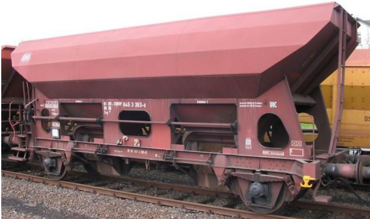
Figure 3: Example of a unit consisting of a (freight) wagon that can be operated separately, featuring an individual frame mounted on its own set of wheels
