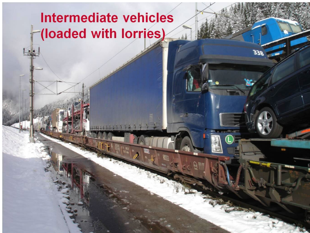
Figure 11 – Example of a unit to carry lorries ('Rollende Landstrasse') – intermediate vehicles
