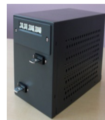
Above : Laminate cell 2000 F / Lithium ion capacitor module
