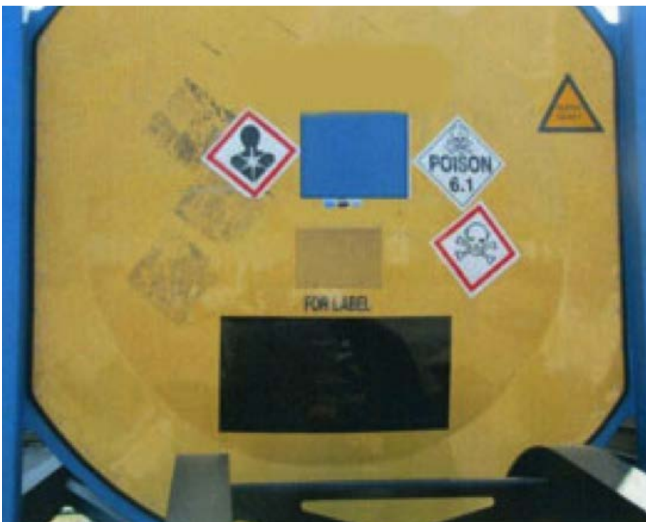
Examples of portable tanks displaying GHS markings in addition to placards of Class 6.1 and Class 3
