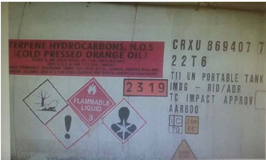
Examples of portable tanks displaying GHS markings in addition to placards of Class 6.1 and Class 3
