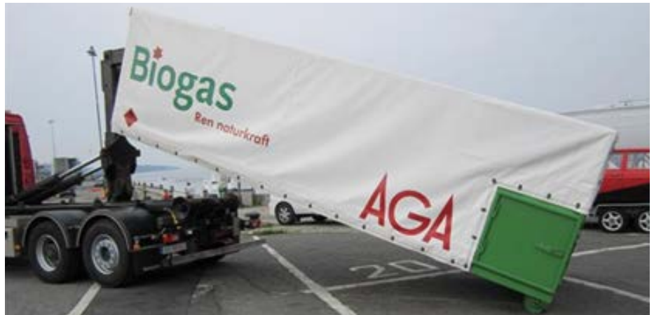
MEGC being unloaded from a lorry using a hook arm lift
