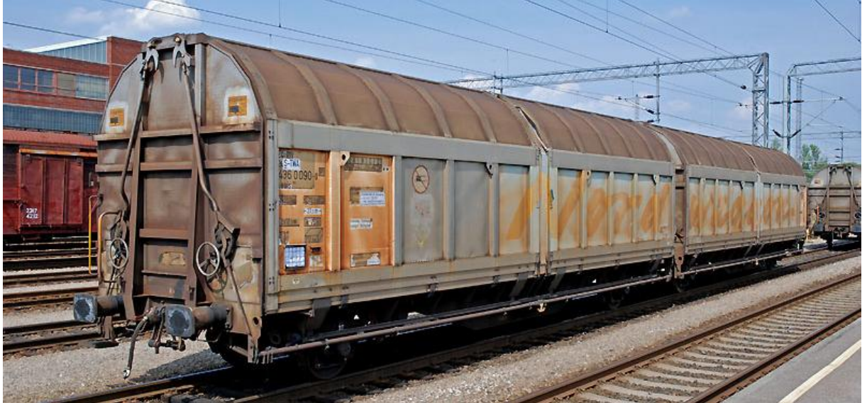
Figure 3: Example 2 of a unit consisting of a rake of permanently connected two elements, those elements cannot be operated separately
