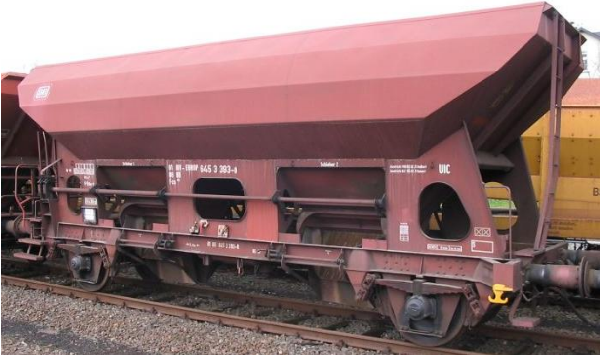
Figure 1: Example of a unit consisting of a (freight) wagon that can be operated separately, featuring an individual frame mounted on its own set of wheels
