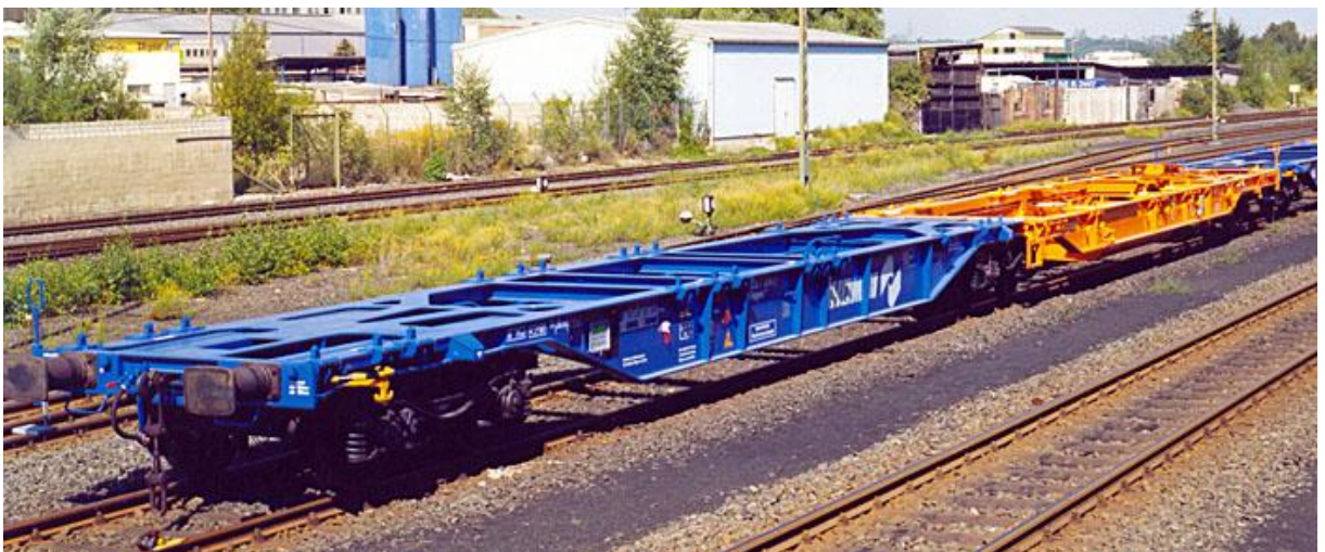
Figure 2: Example 1 of a unit consisting of a rake of permanently connected two elements (blue and orange), those elements cannot be operated separately (articulated wagon)
