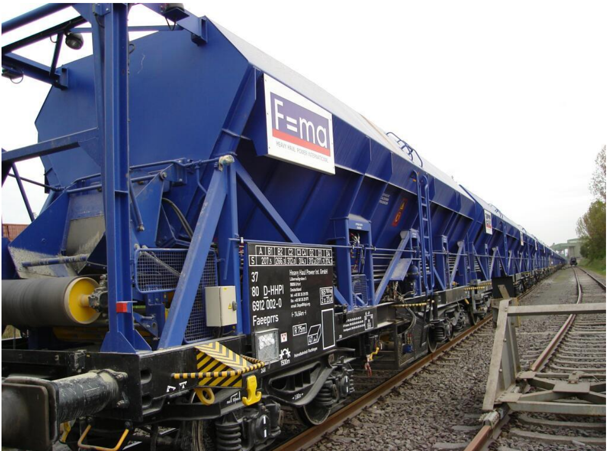
Figure 4: Example 3 of a unit consisting of a rake of permanently connected elements, those elements cannot be operated separately (self-discharging train)
