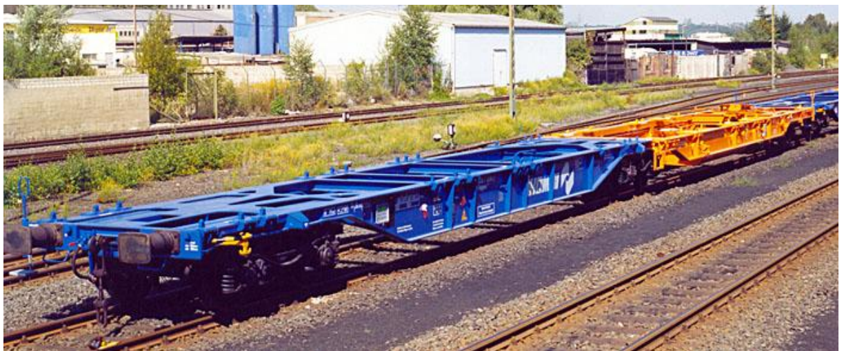
Figure 2: Example 1 of a unit consisting of a rake of permanently connected two elements (blue and orange), those elements cannot be operated separately (articulated wagon)
