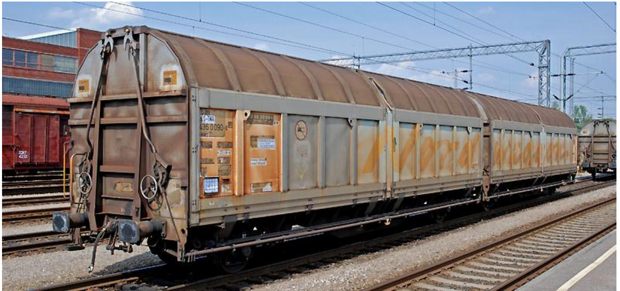
Figure 3: Example 2 of a unit consisting of a rake of permanently connected two elements, those elements cannot be operated separately
