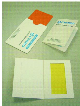
c) Typical paint samples (150 mm × 100 mm) Figure 8 Measurement grids for specimens
