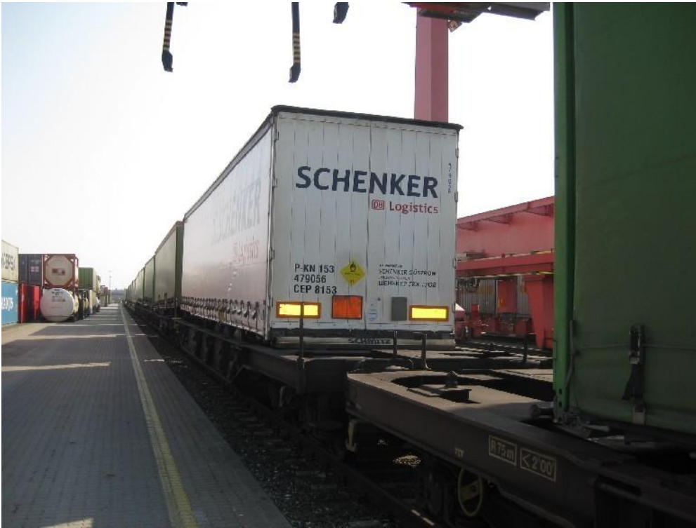
Semi-trailer with marking in accordance with the IMDG Code (placards on four sides). At the rear, additional marking with orange-coloured plates is required!
