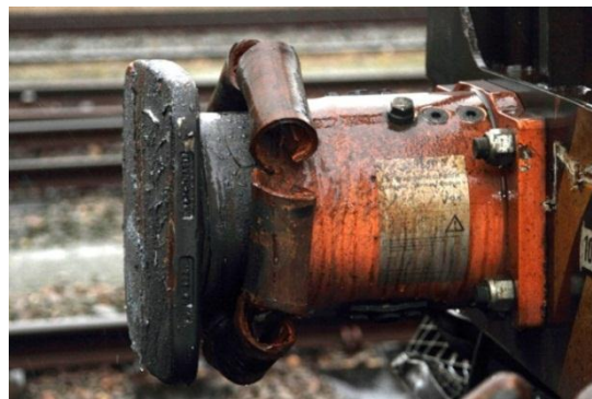
Figure 3: Crash buffer on one of the UN 1268 wagons after the collision in Barendrecht.
