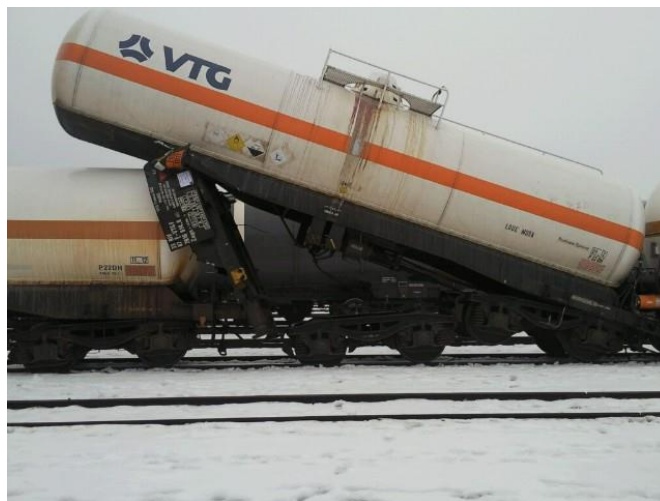
Figure 5: Overbuffering of a chlorine wagon (uncleaned) in Woippy (France).
