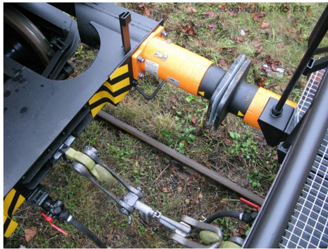
Figure 6: Mutual position of two opposite buffers. Note: the markings (yellow triangles) are indicative of the level of impact during long-time operation: here still as new.
