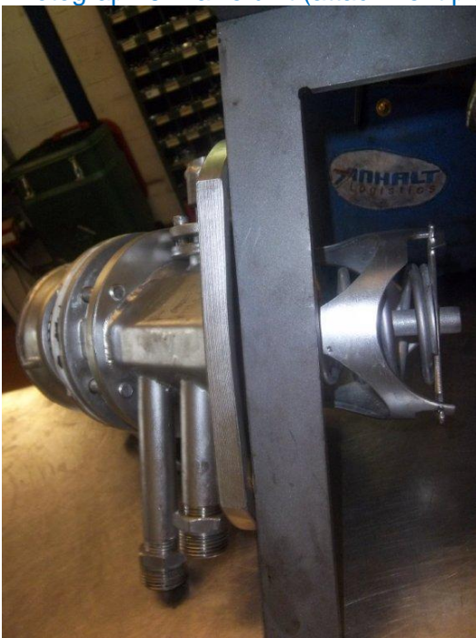
Photograph 5: Valve unit (attachment plate is buckled)
