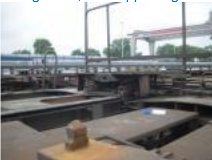
Photograph 9: At the front, an attachment pin for receiving the load unit can be seen and in the background, the supporting frame for receiving the kingpin of the trailer.
