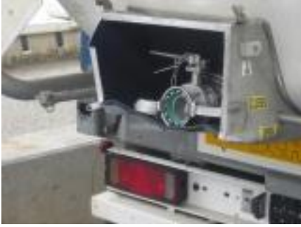
Photograph 3: Close-up of the fittings cabinet bent upwards
