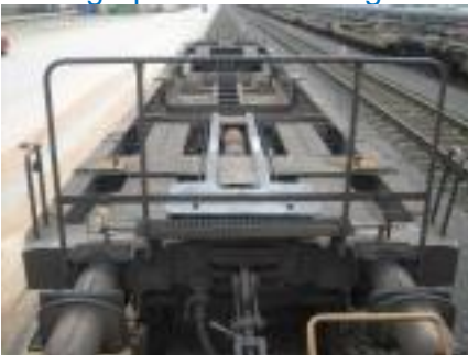
Photograph 9: At the front, an attachment pin for receiving the load unit can be seen and in the background, the supporting frame for receiving the kingpin of the trailer.
