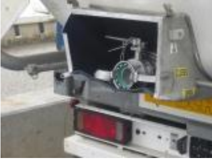
Photograph 3: Close-up of the fittings cabinet bent upwards
