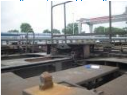
Photograph 9: At the front, an attachment pin for receiving the load unit can be seen and in the background, the supporting frame for receiving the kingpin of the trailer.
