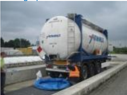
Photograph 2: Tank-container in the drip collector next day
