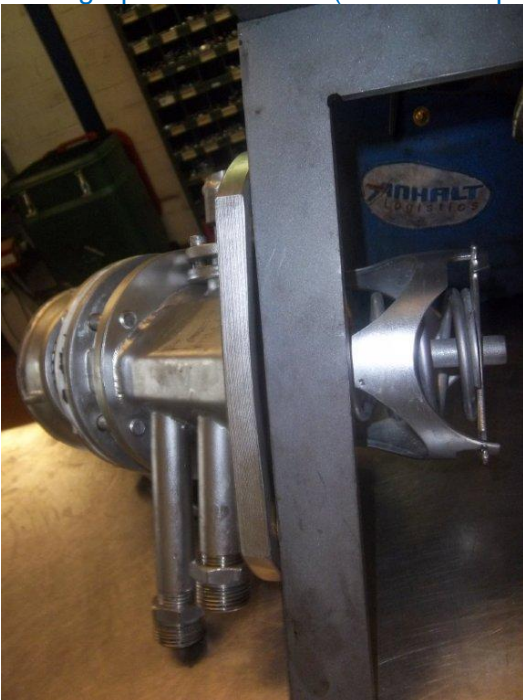
Photograph 5: Valve unit (attachment plate is buckled)
