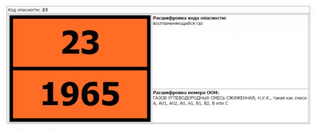
Fig. 3. Explanation of the hazard identification number and UN numbers listed on the orange-coloured plate (for example, the data in Fig. 2).
