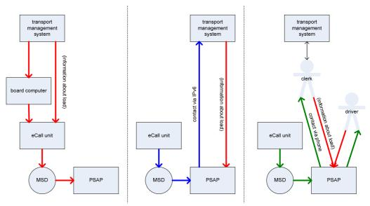
The main goal obviously is getting the information about the dangerous goods at the PSAP. The first and most optimal approach is based on an eCall unit that can be fed with information by either the board computer inside the truck, or the TMS via a remote connections.
