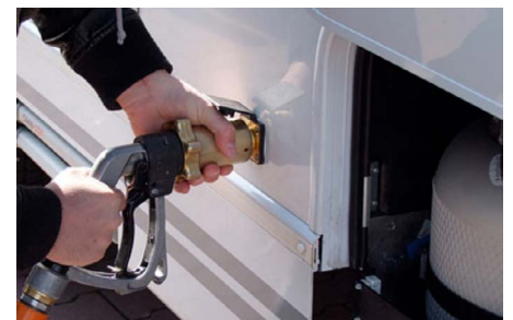
Filling of a fixed LPG cylinder
