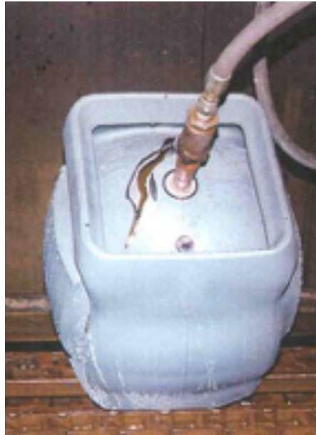
Jochen Conrad Example of a burst test
