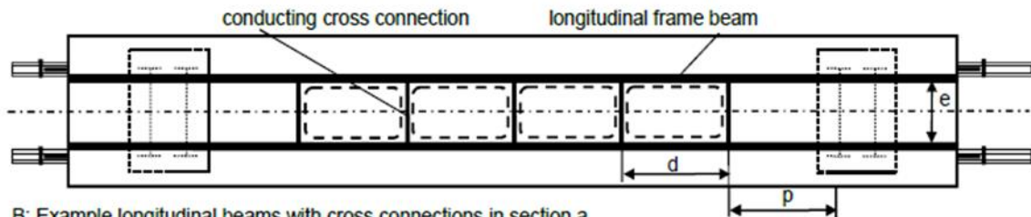
B: Example longitudinal beams with cross connections in section a
