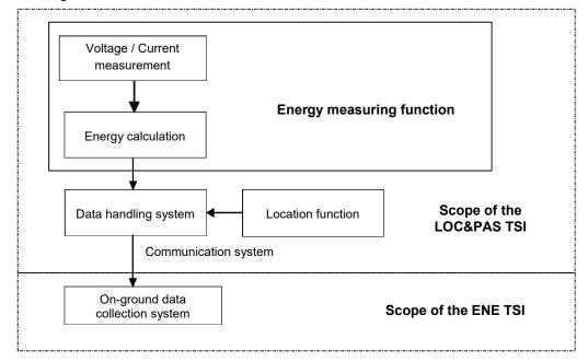
It is permissible to access the data in the EMS for other purposes (e.g. feedback to the driver regarding the efficient operation of the train) provided that it can be demonstrated that the integrity of EMS functions and data are not compromised by this arrangement.
