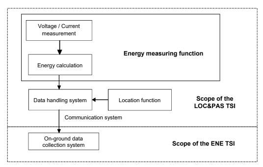
It is permissible to access the data in the EMS for other purposes (e.g. feedback to the driver regarding the efficient operation of the train) provided that it can be demonstrated that the integrity of EMS functions and data are not compromised by this arrangement.
