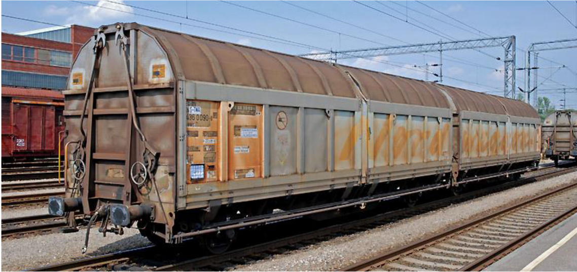
Figure 5: Example 2 of a unit consisting of a rake of permanently connected two elements; those elements cannot be operated separately
