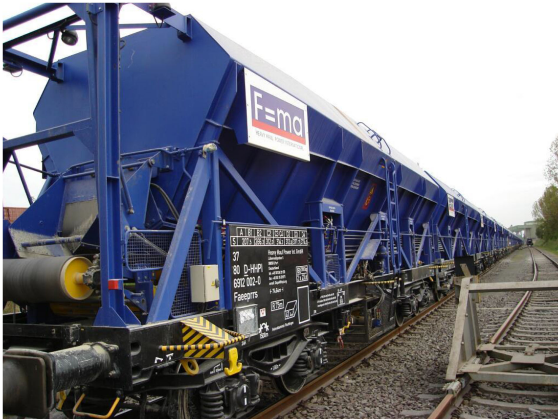
Figure 6: Example 3 of a unit consisting of a rake of permanently connected elements, those elements cannot be operated separately (self-discharging train)
