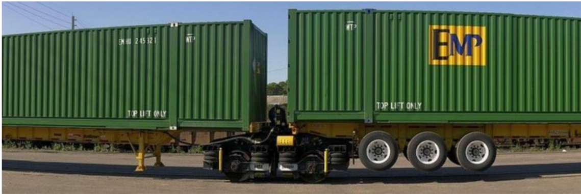
Figure 7: Example 1 of a unit consisting of separate rail bogies connected to compatible road vehicles
