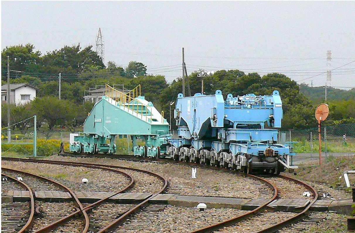
Figure 2: Two examples of vehicles that increase their length in loaded configuration and their payload is part of the vehicle structure (in unloaded configuration)
