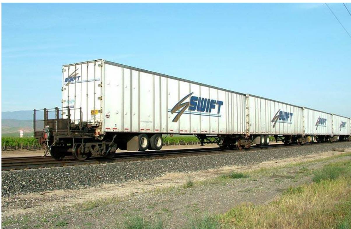
Figure 8: Example 2 of a unit consisting of separate rail bogies connected to compatible road vehicles
