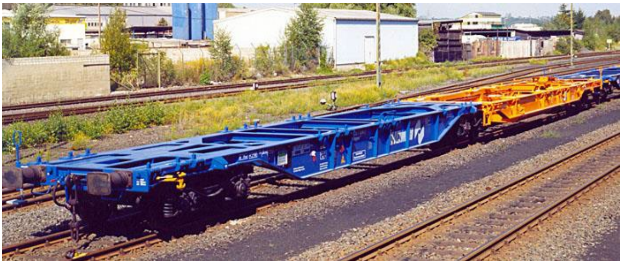
Figure 4: Example 1 of a unit consisting of a rake of permanently connected two elements (blue and orange), those elements cannot be operated separately (articulated wagon)
