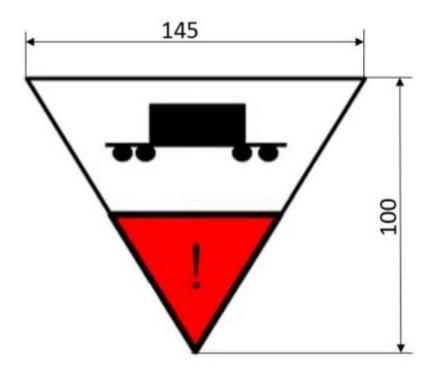
NB: Fly or hump shunting and buffing is not permitted when the wagon is loaded. Shunting may be performed without restriction when the wagon is empty.
