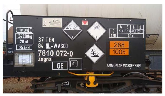
4. For compressed gases filled by mass, liquefied gases, refrigerated liquefied gases and dissolved gases the load limits referred to in 6.8.3.5.7 depend on the gas loaded in the tank. Therefore, in the case of multi-purpose tanks, the name of the particular gas being carried shall be stated, together with the load limit on the same folding panel.
