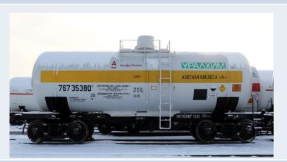
application of the materials providing working capacity at temperatures down to - 60°C regarding tankwagons of 1520 mm track gauge is taken into account (6.8.2.1.8, 6.8.2.1.10, 6.8.3.2.20)
