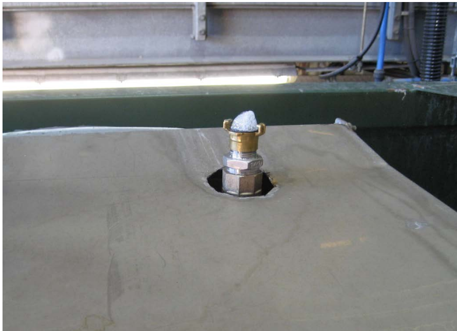
Picture 4: Gas displacement nozzle with part cut out of dome case cover
