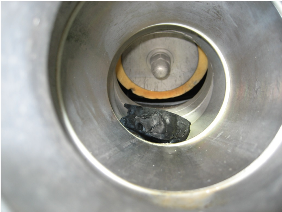
Picture 1: Foreign body in bottom outlet
