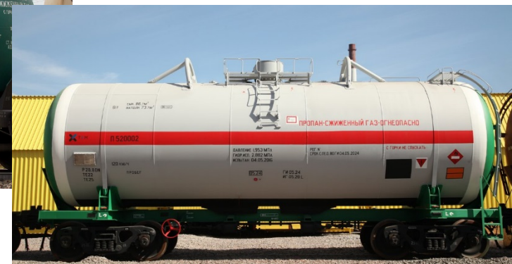
Tank-wagons equipped with fittings protection equipment, intended for the carriage of liquefied gases
