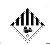
(No 9A) Symbol (seven vertical black stripes in upper half; battery group, one broken and emitting flame in lower half): black; Background: white; Figure "9" underlined in bottom corner
