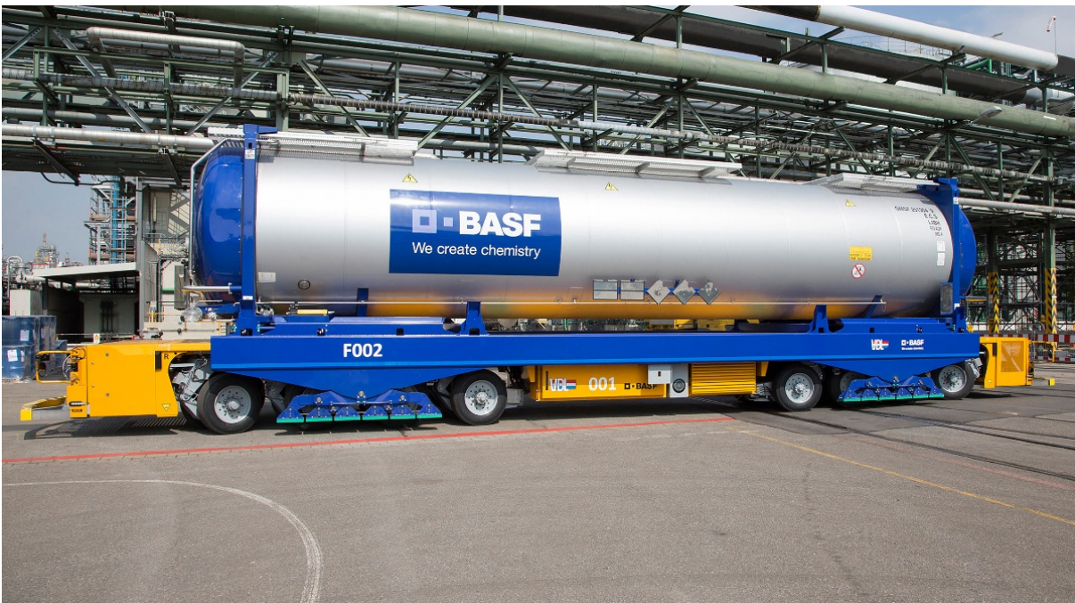
Picture 2: Within the industrial site, the B-TC can be carried by automated guided vehicles.
