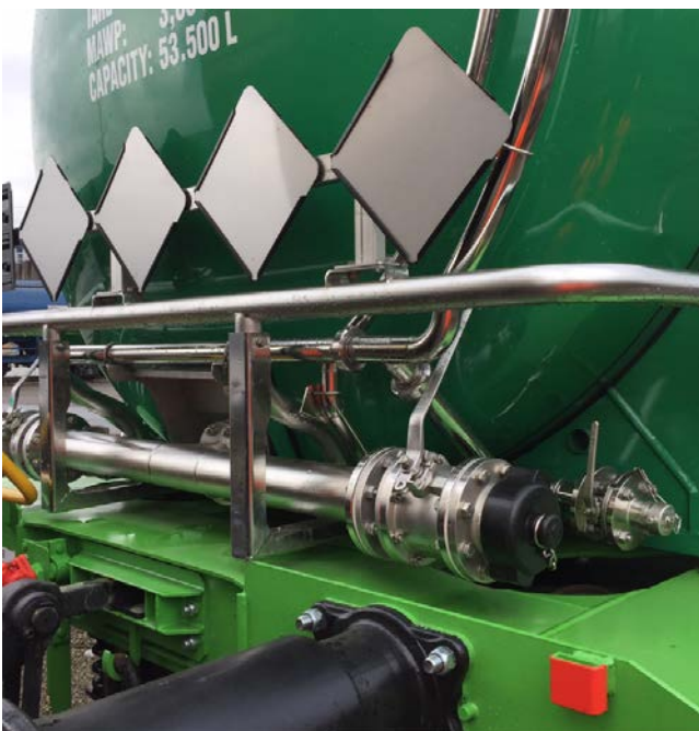
Picture 4: Close-up view of tank end with service equipment above buffers (SBB Infrastruktur, 08.11.2017)
