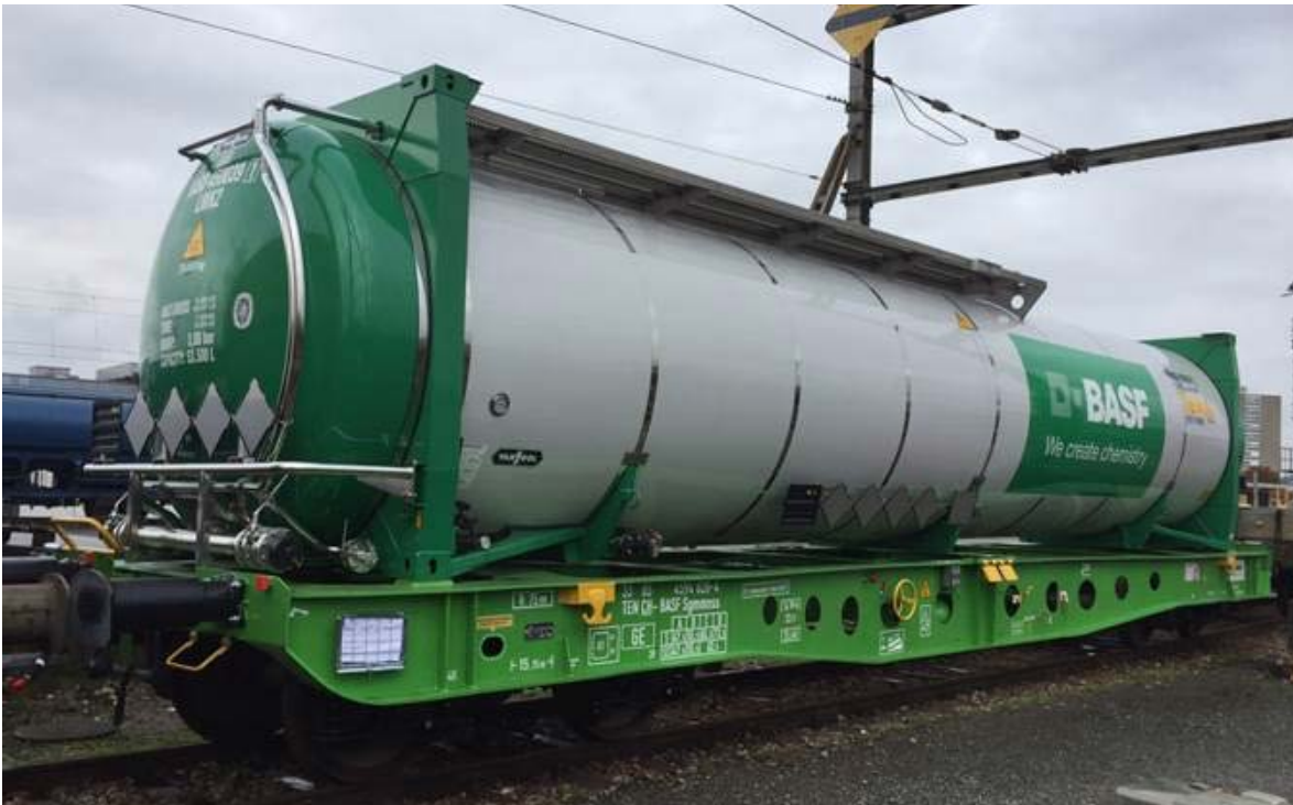
Picture 3: B-TC on specially designed carrying wagon (SBB Infrastruktur, 08.11.2017)
